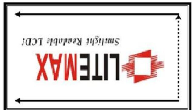
Fig. 2 Reverse scan (pin 28, UD/LR = Hight )
