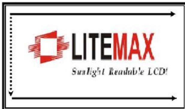
Fig. 1 Normal scan (pin 28, UD/LR = Low )
