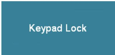
To release the OSD lock, press and “**right >**” and “Menu”. The below icon will appear on the center of the screen for 8 ~ 9 seconds. Now all OSD keys are active again.
